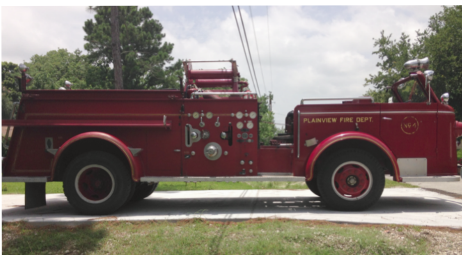
Delivered January 1951. 750 GPM pump with a 12 cylinder gas engine, series G, 491 CUID, ex-Plainview
