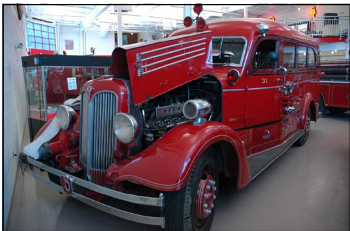
In 1936, the City of Detroit placed four Seagrave Safety Sedans into service. Detroit would eventually purchase 67 of these. The fully enclosed design allowed firefighters to sit inside the rig rather than standing on running or tail boards. They were powered by V-12 engine and could pump up to 1000 GPM
